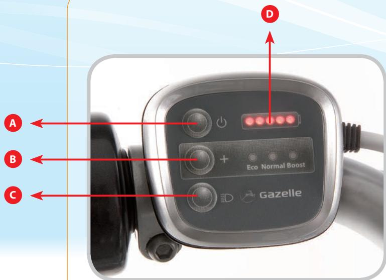
The display is on the left hand side of your handlebars and cannot be removed. A summary of the various indications on your display is given below.
