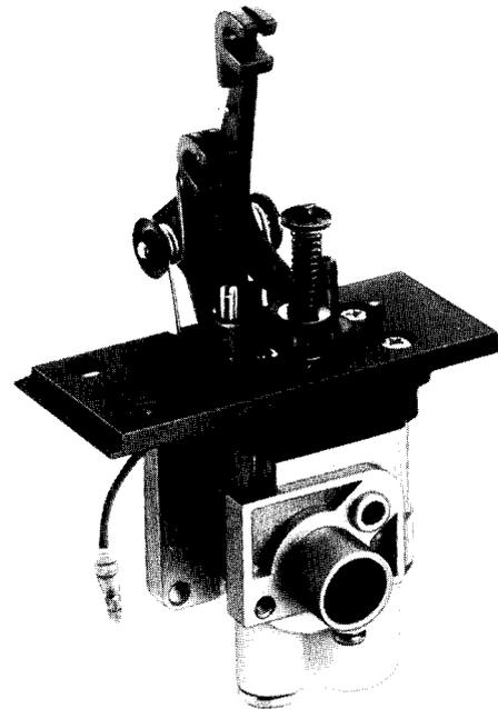
stem. When the engine is started a particularly high vacuum occurs at the fuel outlets, which gives the necessary fuel enrichment for starting. The starting valve is operated with the starting lever (23). A lug on the valve pushes the lever (34), thereby operating other parts of the carburettor.
