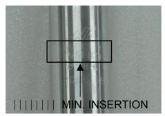
Take heed of the maximum height markings (MIN. INSERTION) on the tube of the seat.
