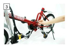
Coincide the locking holes and insert the safety pin to engage the front and rear frame assembly securely.
