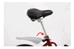
4. Tighten the clamp lever.
