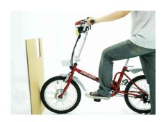
2. Then, press the main switch to either left (I) or right (II) position while depressing the pedal.
