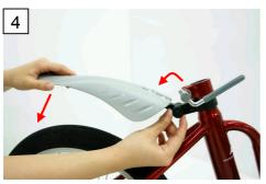
Lower the mudguard by loosening the tighten knob.
