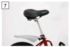
Install the saddle and adjust it to the desired height and then tighten the clamp lever.
