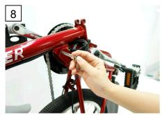
Insert the safety pin into the locking holes to engage the front and rear frame assembly.
