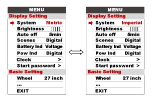
8.2 Brightness : Press Up / Down button to change the brightness of the backlight, I is
