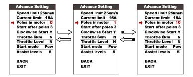
**8.15 Start after poles** : How many poles (speed sensor) need to be detected by controller before starting motor. Default value is 3.
