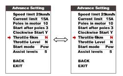
**8.18 Throttle Level** : This parameter is functional when Throttle 6KM set N, Press UP/DOWN will change Y/N, N represent Throttle start max speed, Y represent throttle's speed is accorded to the assist level.
