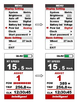
\* This data represent power output of the battery (not motor).
