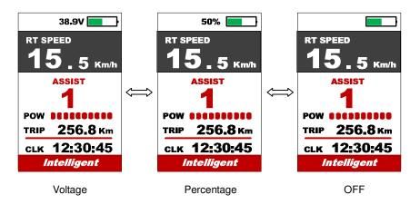
8.6 Pow Ind : Press UP/DOWN button to change the Power indicator, Analog / Digital.
