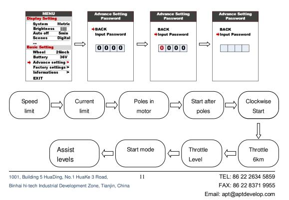
**8.12 Speed limit** : Press UP/DOWN will change speed limit, range 10km/h~45km/h. Default value is 25km/h.
