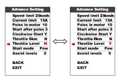
8.19 Start mode : Pow/ECO/STD represent Power/ECO/Standard, Power mode means use maximum current when speed up (default), ECO mode means use minimum current.
