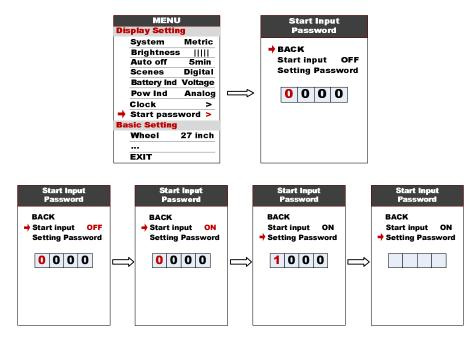
You need to input the right password before start with 30 seconds, display will power off automatically if the password was wrong.
